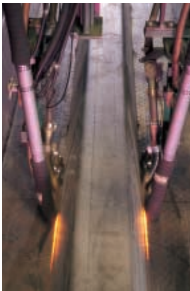
Automated submerged arc welder provides continuously welded joints.
