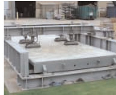
Tandem axle load simulator empirically validates the design.
